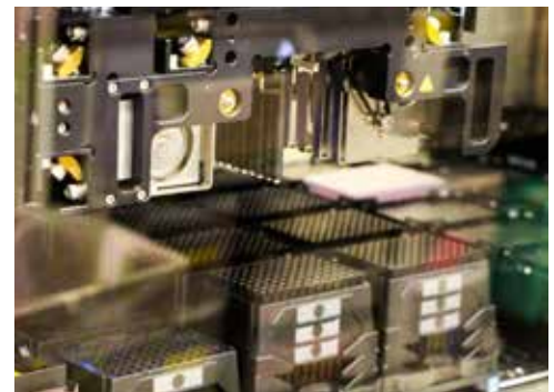
The NYSCF Global Stem Cell Array automates the production of hundreds of stem cells from patients in tandem
